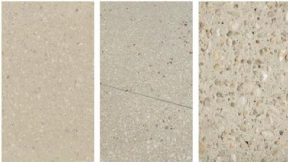
Figure 14: In-situ decorative surfacing etch and aggregate finishes ranging from the 0.5mm (left) to approx. 3mm (right)
